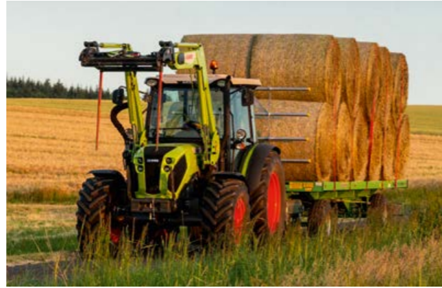
The design of the mounting brackets allows a CLAAS front loader to be retrofitted at a later date.
