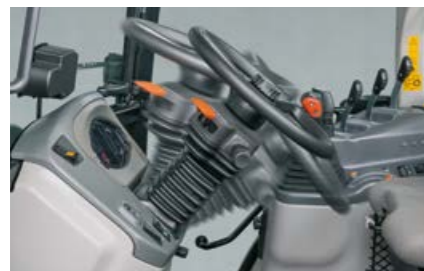
You can vary the tilt and height of the adjustable steering column for optimum comfort
