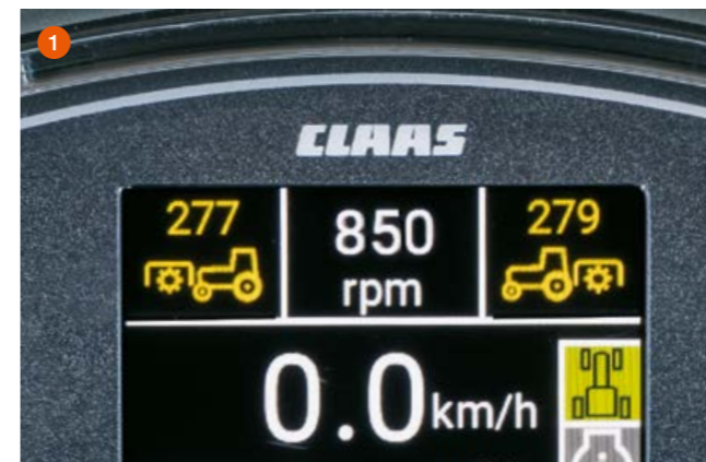
1 The digital speed indicator for the front and rear PTO means that you're always working at just the right speed
