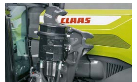
FITLOCK system for rapid attachment/removal and MACH quick-release coupler for electric and hydraulic connections
